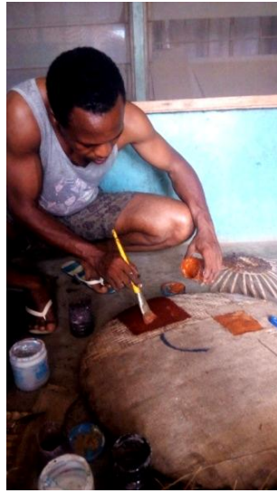
Plate 5. Ukwa, Job N. Exploring the possibility of using gumming technique to fasten jute fabric on woven cane tray. Photo by Okechi Benard
