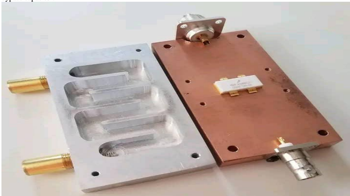
Figure 7. Mechanically design high power 48-V LDMOS
