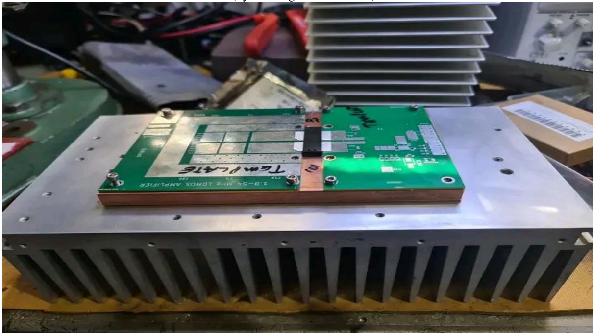
Figure 14. Construction of RF LDMOS
