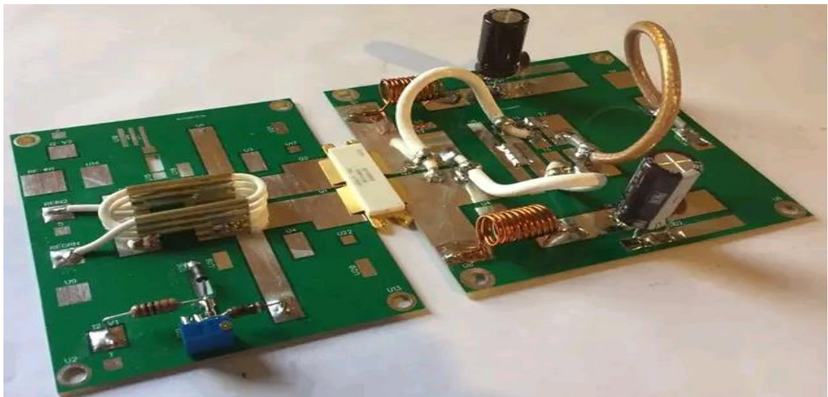
Figure 16. Photograph of RF FM LDMOS Pallet Amplifier
