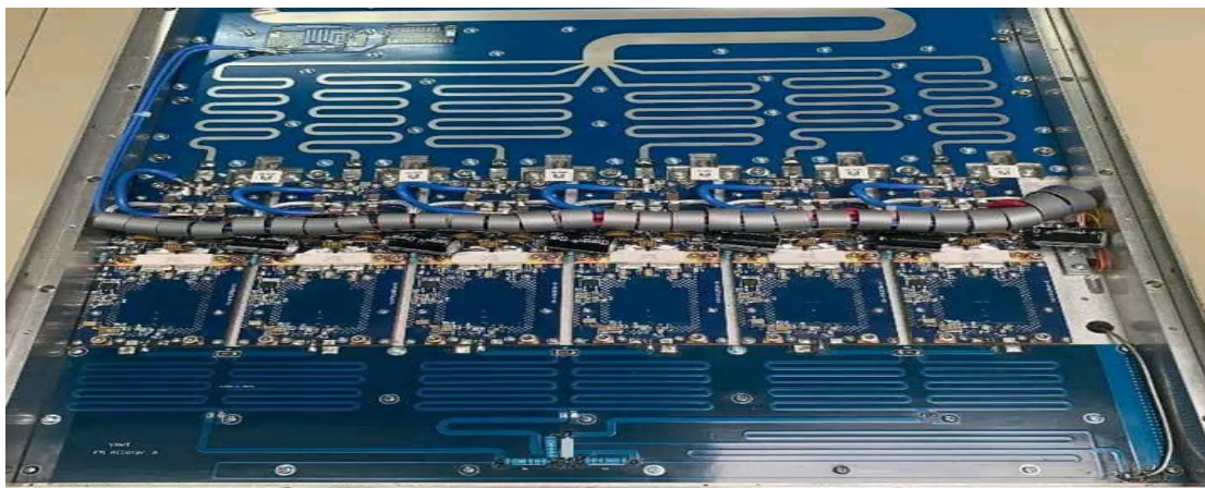
Figure 8. Photograph of combined amplification using Strip lines
