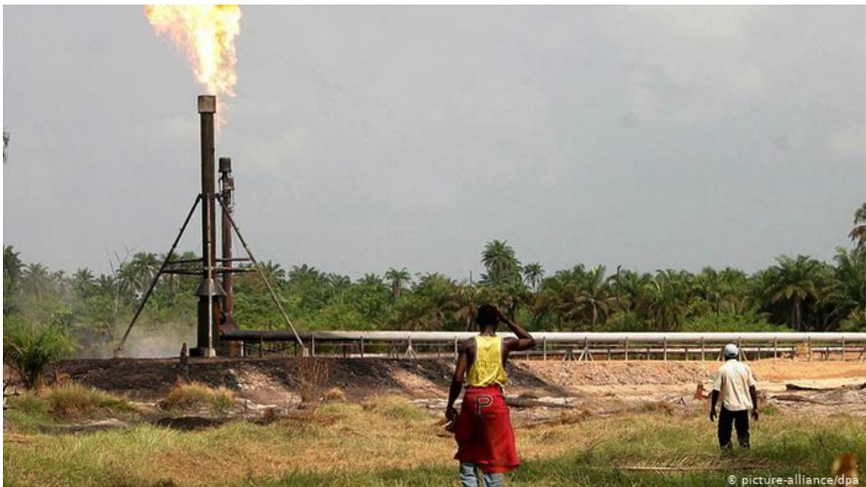
The above picture shows the method adopted by oil companies to get rid of waste gas released through drilling by oil industries. This flow station is located less than 100 meters (109 yards) from a residential area in a small village near Ekpetiama Yenagoa in the Niger Delta region. The burner close to this area has resulted in respiratory problems for the residents of the area.
